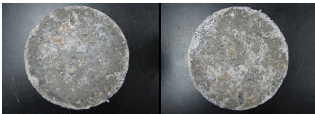
Figure 3 Interface morphology of L mixture after bond strength test. [Color figure can be viewed in the online issue, which is available at www.wileyonlinelibrary.com ].
